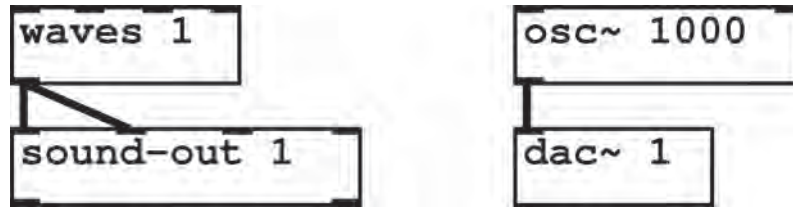
Figure 1: The different procedures in Abunch (left) and Pure Data (Pd) (right). In Abunch the argument (the number after the object name) always refers to the preset system. In Pd there are more options: '1000' refers to the frequency of the oscillator 'osc~' object and '1' to one audio hardware output of the digital-to-analog converter 'dac~'.
